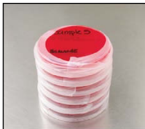
Wrap sample plates in parafilm
